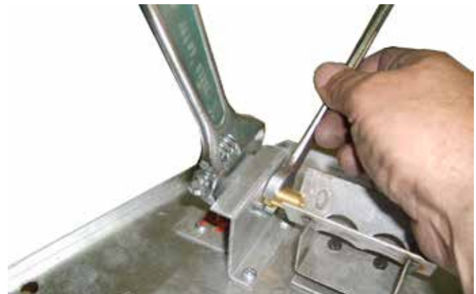
Fig. 83 Use two wrenches to avoid damage to manifold.
